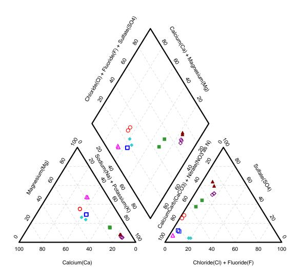
Figure 4.22 Piper Diagram Comparing Task 1 Primary WAter Quality Sample Results with QA/QC Sample Results.
