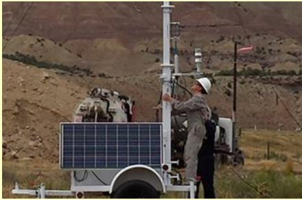
VOC monitoring in Garfield County includes Hazardous Air Pollutants (HAPs) such as the BTEX compounds (Benzene, Toluene, Ethylbenzene and Xylenes)
